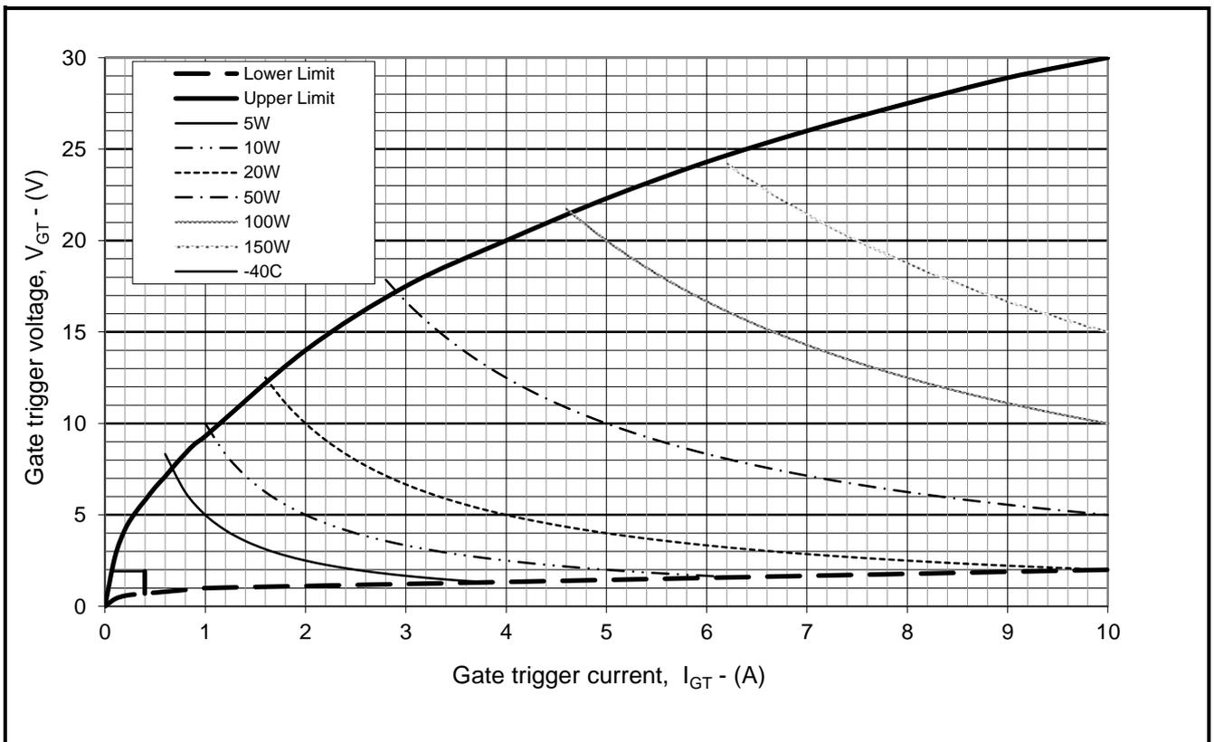
Fig. 15 Gate characteristics
