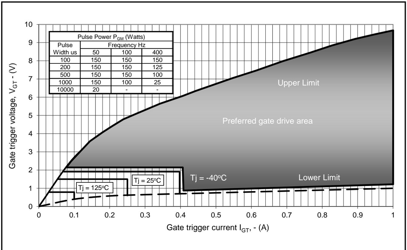
Fig14 Gate Characteristics
